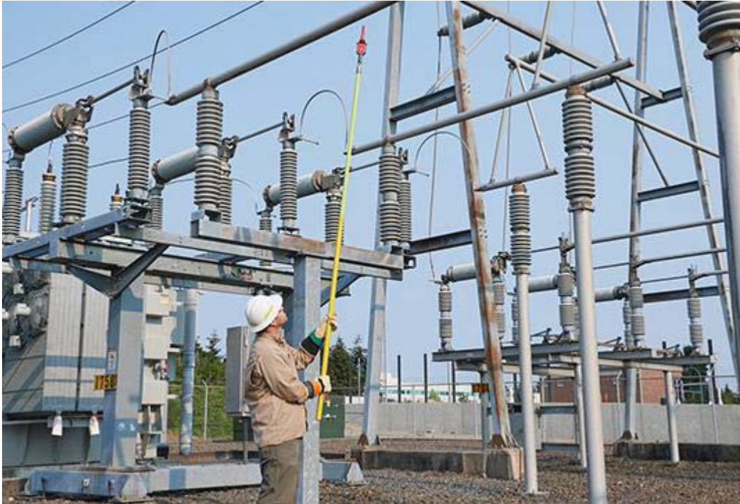
The TIC 300 PRO High Voltage Tester: MSHA certified and intrinsically safe
